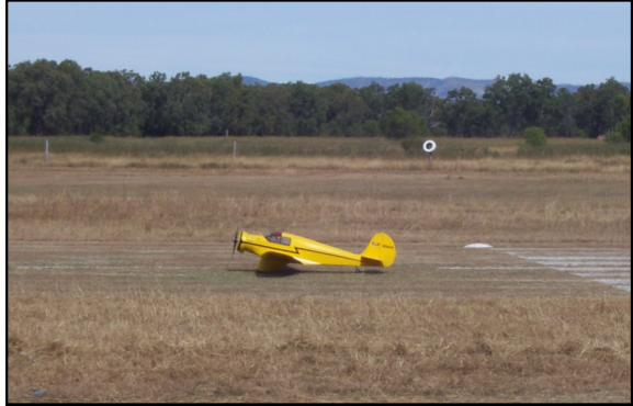
Above: Ray Thompson's (Mackay) Aeronca LB. This model has a 122" Wingspan and powered by a super tiger 3000.
